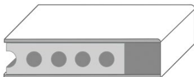
PERFORATED CHIPBOARD filling
