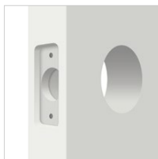
REBATE preparation for standard doorknob with 2 3/8"
